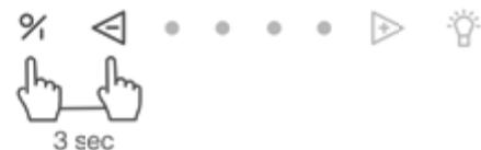
The function can be switched on by pressing the and keys at the same time for 3 seconds.
